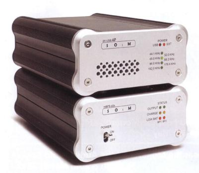
he awkwardly named SOtM is from Korea. It is an asynchronous convertor that accommodates 44.1 and 48k sample rates and their multiples all the way up to 192kHz, with up to 24bit resolution, so this convertor ticks all the boxes. It comes with a USB driver disc for Windows (XP/SP3, Vista/SP2, 7), or will work with Mac OS-X 10.6 (Snow Leopard) onward. Data rate must be set in the Advanced tab of the Sound control panel in Windows.
